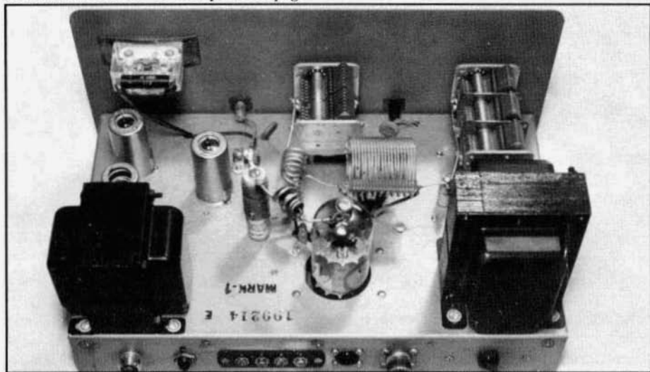
Rear View of the HT-40. The 6DQ5's socket is mounted 1-1/4" below the chassis to minimize the height of the front panel.
