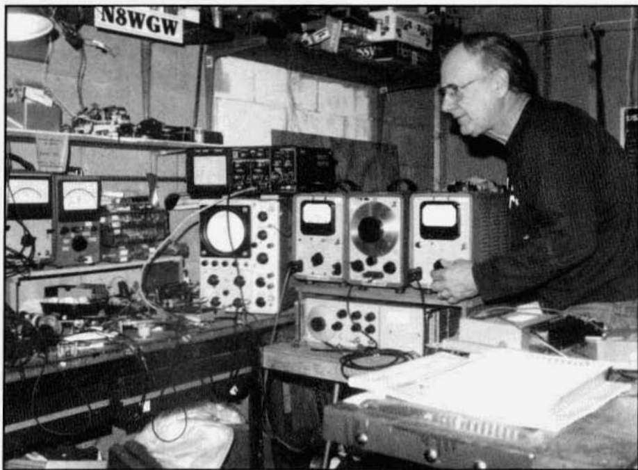
Another view of Kurt Miska's not-too-tidy workbench. He's adjusting one of his H-P 400D AC VTVMs, two of which flank an H-P 200CD extended range oscillator. Under this threesome is an H-P 3300A function generator.
