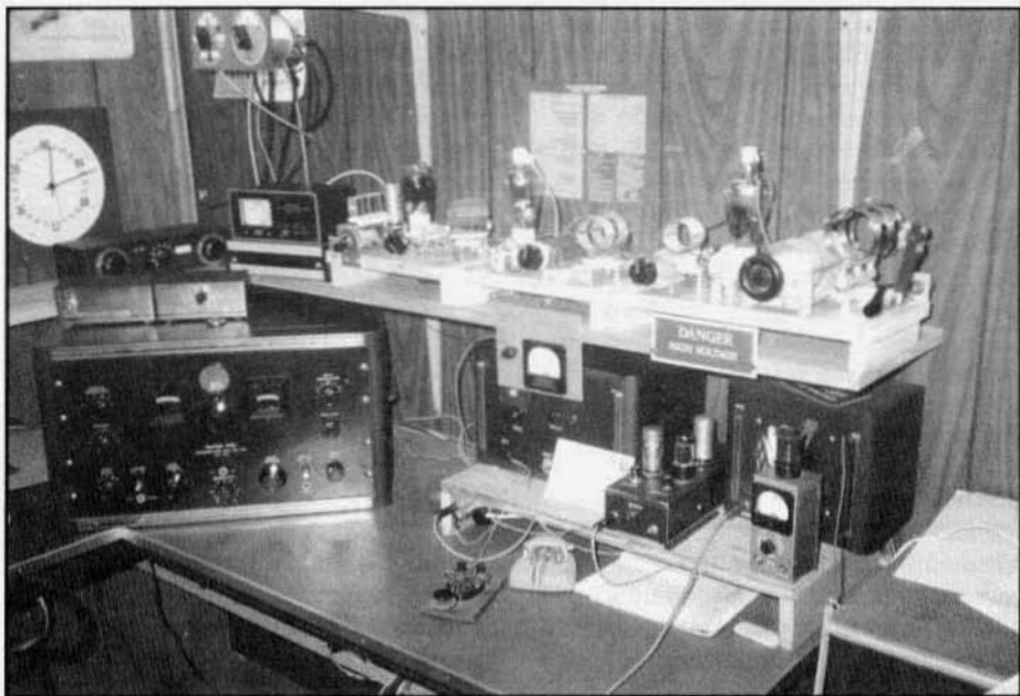
WØREP's vintage station. The top shelf holds the Taylor transmitter. On the table at the left is a Hammarlund SP-200 receiver. The platform on the right holds the VFO, keyer and receiver speaker.
