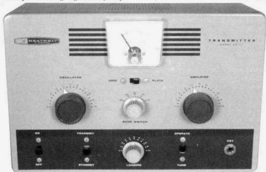
HX-11, 6-band CW transmitter, one of the least known and rarest of Heathkits transmitters.
