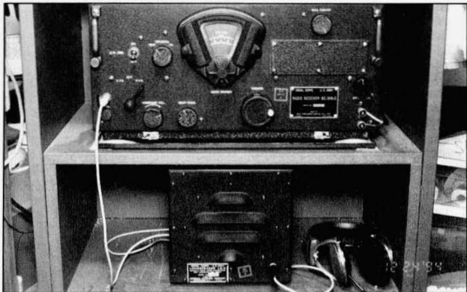
The finished LS-3 below my BC-348-O. The Stancor matching transformer is "hidden" behind the LS-3.
