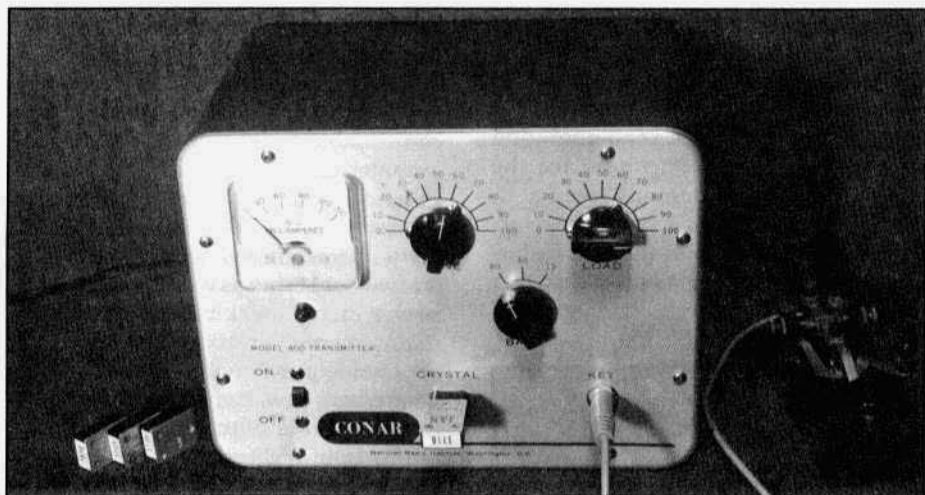
Conar 400 transmitter with xtals and key; ready to go on the air.
