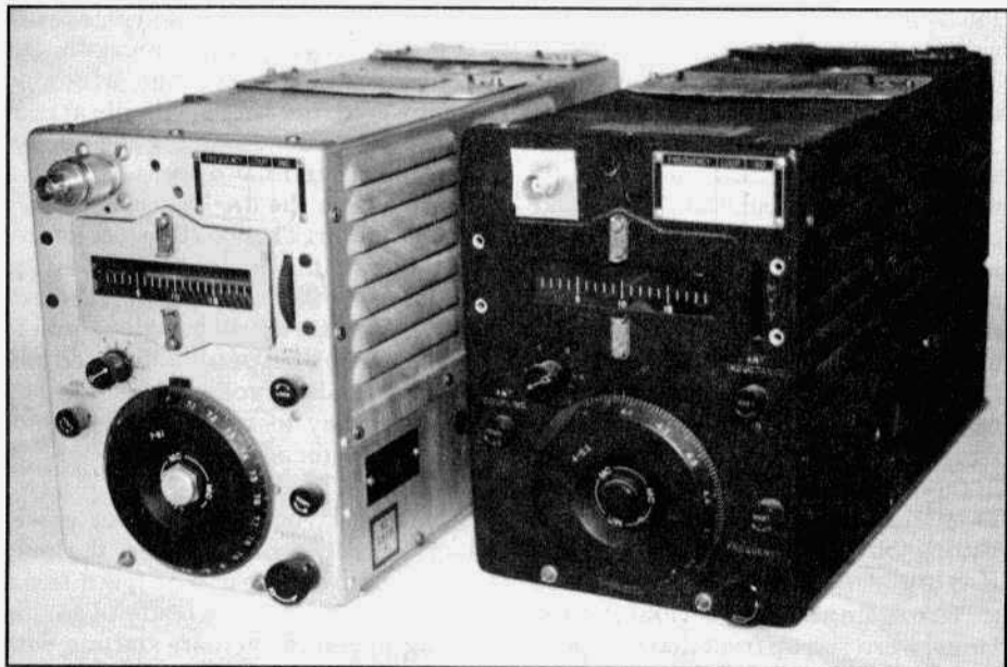
Command Set Transmitters. Left a Western Electric BC-459, 7 to 9.1 Mc. Right a CBY-52209, Navy BC-457, 4 to 5.3 Mc, pulled down to cover 80 meters.
