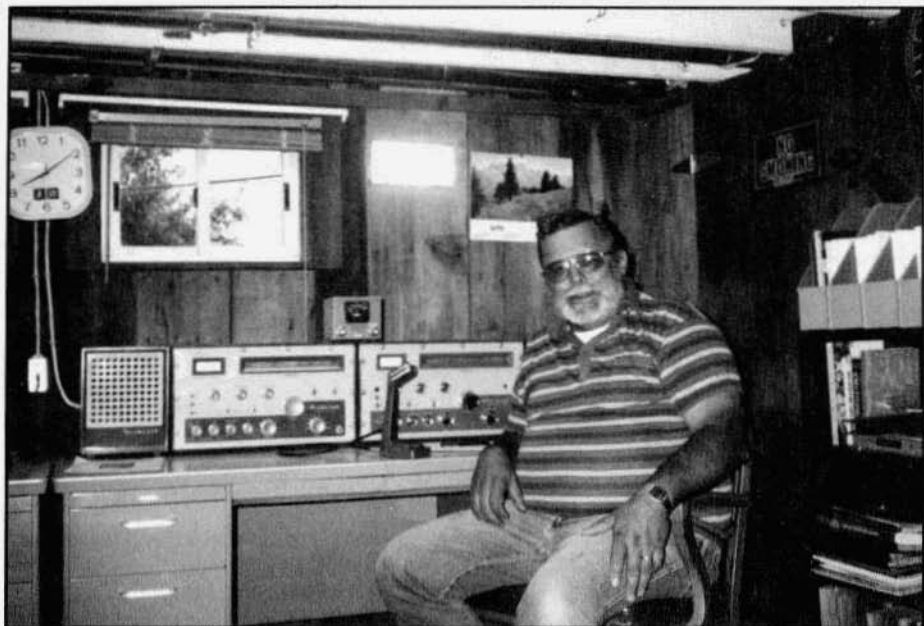
Ken Burrough, NEØC, in his ham shack. Note the pristine Heathkits; the Apache (TX-1) and Mohawk (RX-1).
