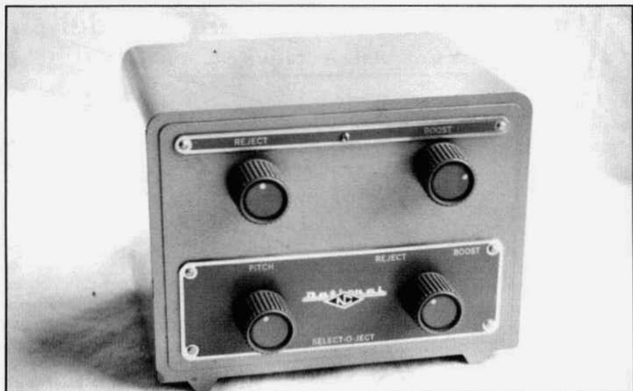
The National Select-O-Ject, one of the first audio filters.
