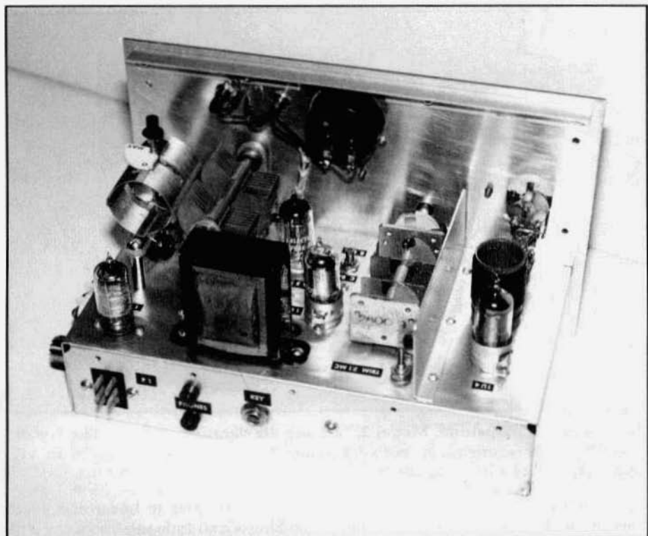
Rear View: Oscillator tank coil is at left.
