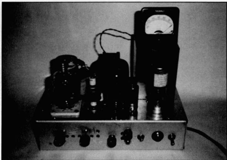
A simple, monoband transmitter using a low-cost 829B final.
