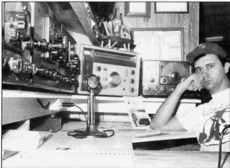
Bill Jensen, WØWI, at his Johnson operating position. The upper shelf holds a Viking II, 122 VFO and SX-125 with matching speaker. Photo courtesy of James Jensen, WAØLEU.
