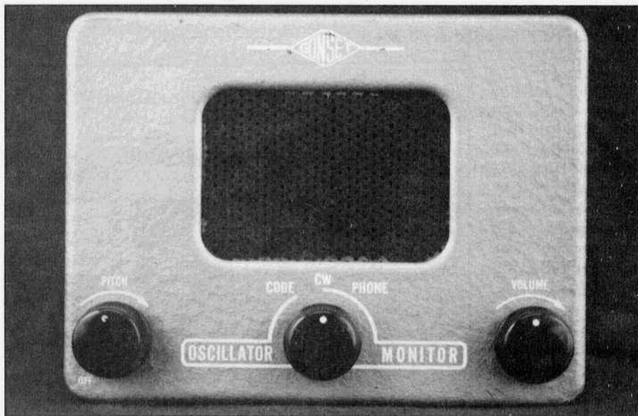
Front of Gonset Monitone. Red flocking on the speaker grille and corresponding red knobs highlight the front wrap-around panel. Dimensions are 6-3/4" wide, 5-1/4" high, 4" deep.
