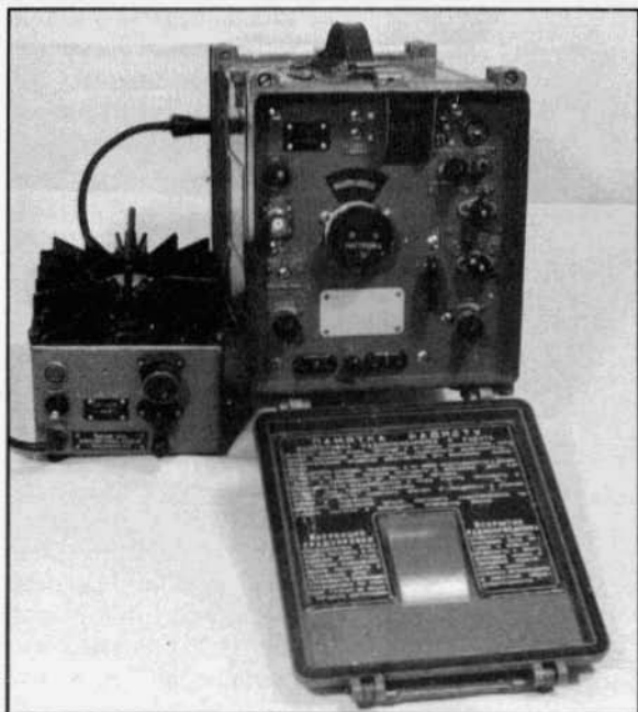
R-326 receiver with open front cover. The AC power supply is on the left.
