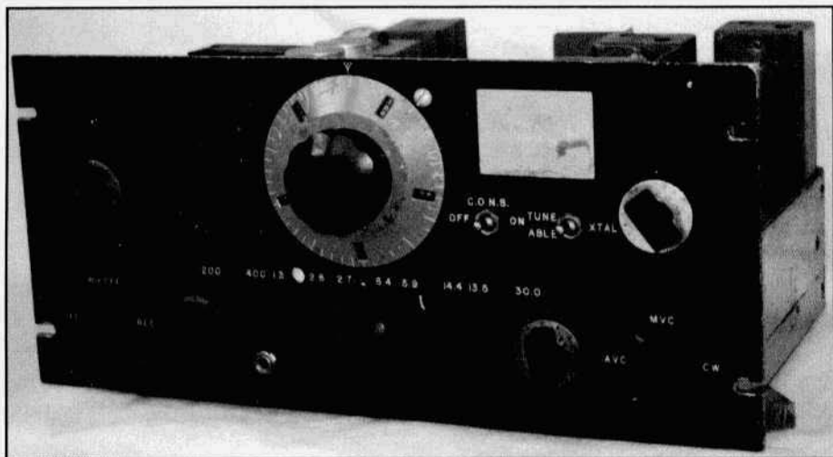
The Mystery Receiver, an NC-100 spinoff. White dot indicates it's on the 1.3 to 2.8 MHz band.
