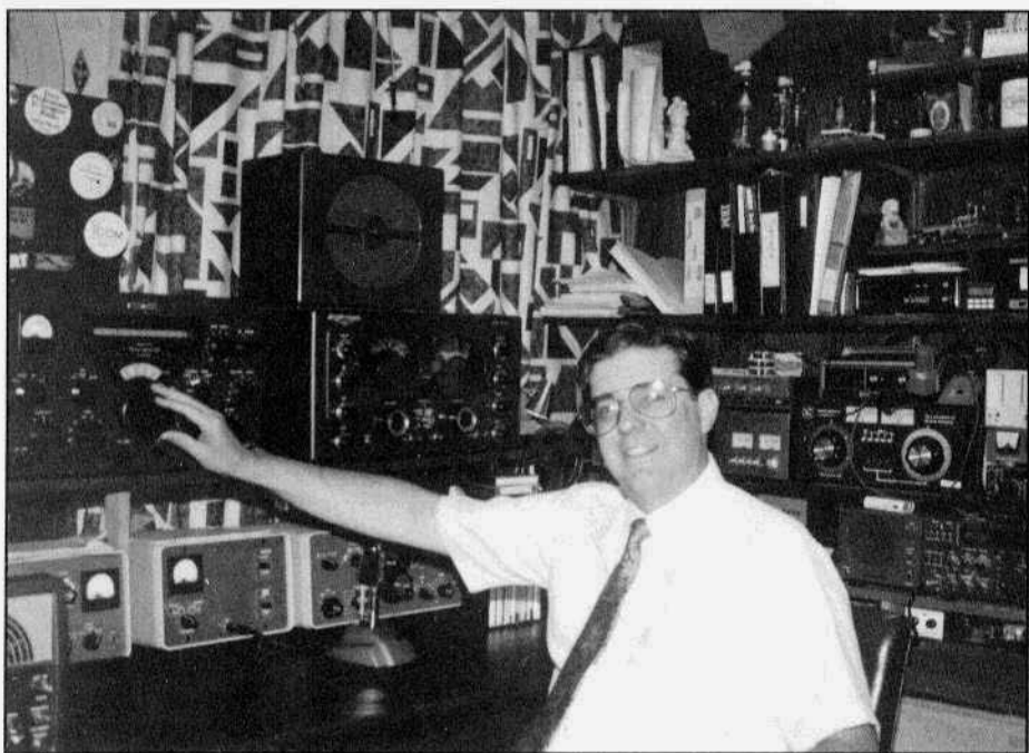
Brian Davis, W9HLQ, in his hamshack. The receiver he's tuning is a Collins 75A-4. The receiver to the right is a National NC-183D. Below those two receiver is a Collins S-Line.
