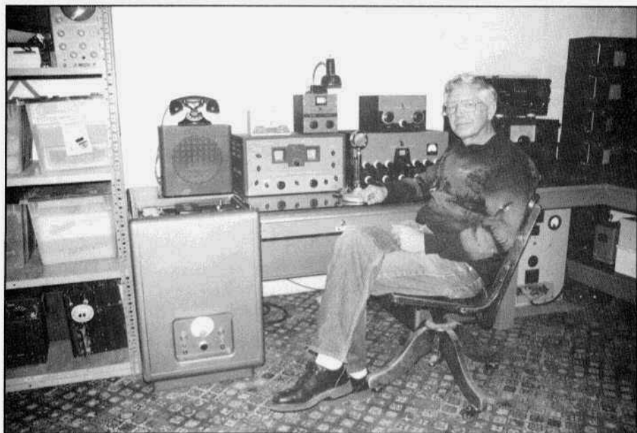
Jerry Fuller, W6JRY, at his AM operating position; Desk KW, HQ-129X and Viking II.
