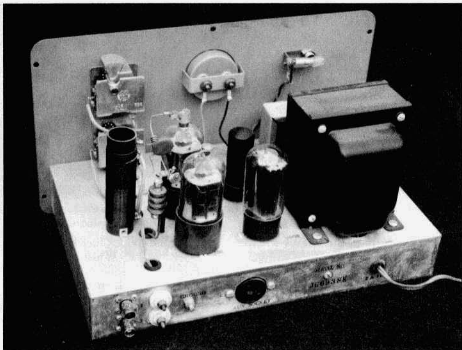
An inside view of JG 69388K. Note the metal back on the meter and the two output terminals for the PI-L match. The final tubes are 807W's.
