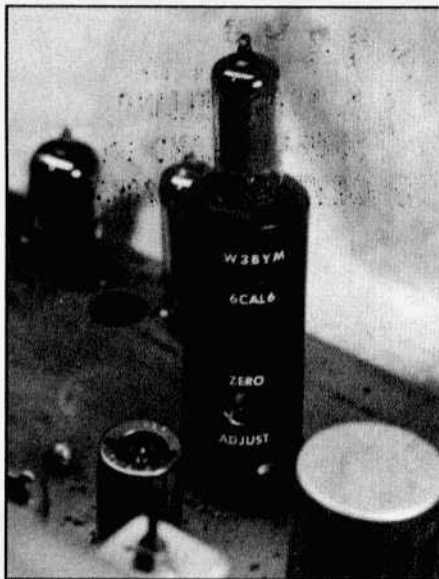
The '6CAL6' calibrator installed in the author's NC-300.
