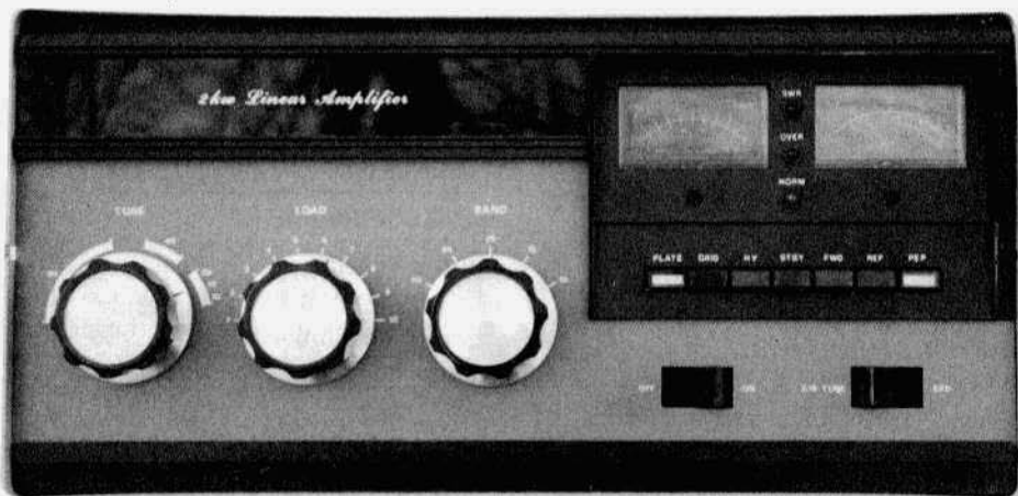
Front panel of the SB-240 linear amplifier.
