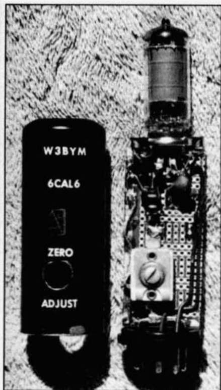
The shell of the 6L6 removed showing construction of the calibrator.
