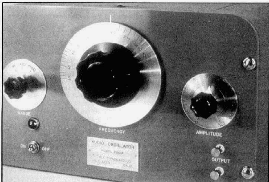
Hewlett-Packard's first product, an audio oscillator, was used by Walt Disney Studios to test sound equipment for the movie "Fantasia."
