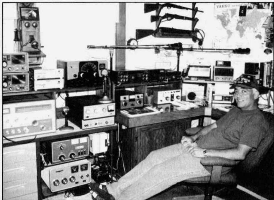
George Folse, KB5WWO, at his operating position. Some of the gear in the photo includes a TX-1 (on the desk, on the left) and a Ranger (same desk, upper right). The amplifier in front of the Ranger is a Gonet GSB-201.
