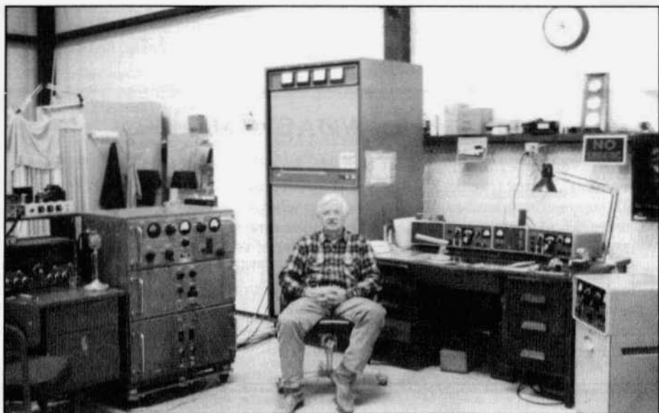
Wes Minear, W7UO (ex W9UO) in his ham shack. The transmitter on the left is a T-368. The unit against the wall is a Gates BC1G that Wes uses on 160. A complete S-line station sits on the desk with a 30S-1 amplifier next to it on the floor.
