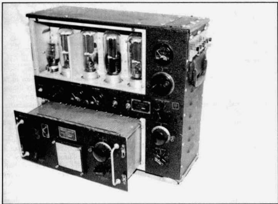
The BC-191 transmitter with front panel removed and tuning unit partially removed.
