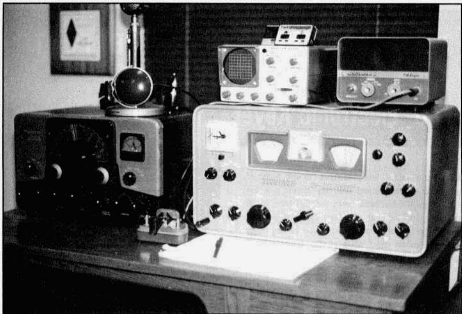
The HA-1 keyer on top of a HQ-170 receiver. The transmitter on the left is a Johnson Viking Ranger.
