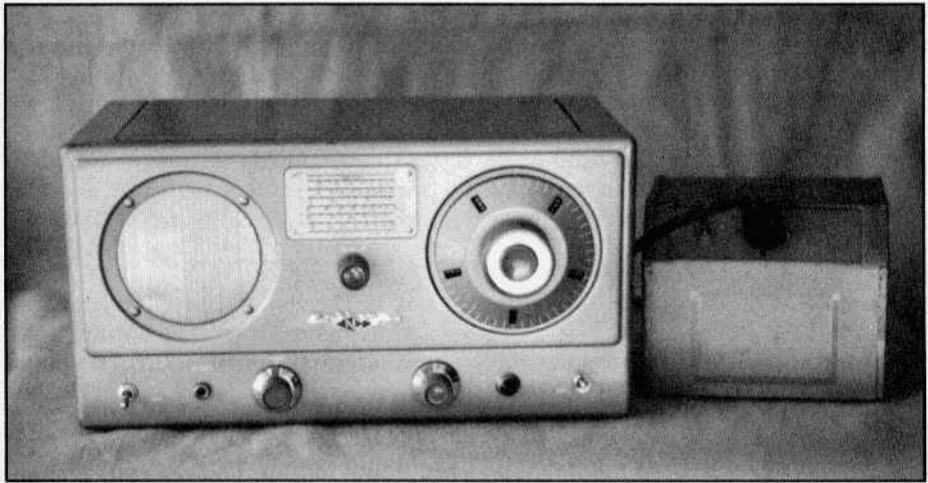
Figure 1. The HFS receiver with 'doghouse' power supply. Note the built-in speaker. Photos by Clyde Watson.
