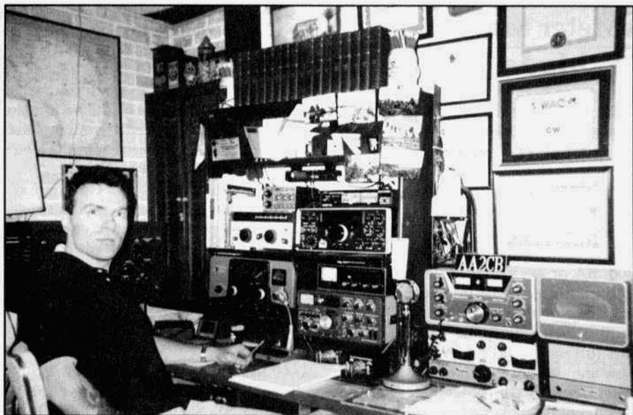
Rosario DiPeri, AA2CB, at his operating position. His station consists of both vintage and modern gear. Some of the vintage gear includes: a 75A-2 behind him; a Johnson Ranger in front of him to the left; a Hallicrafters SR-500 (under the callsign) and a Swan 240 under the SR-500.
