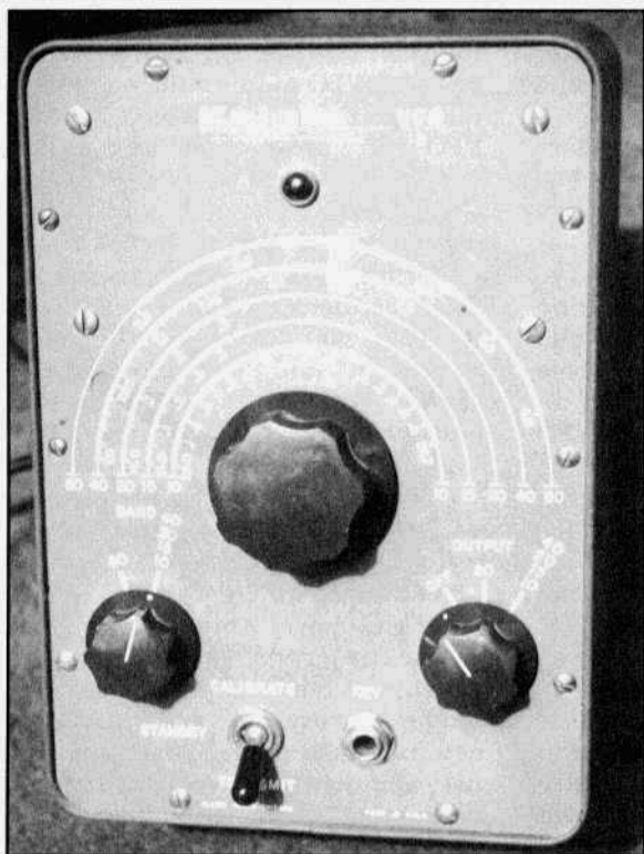
Allied Radio's Knight-kit V-44 VFO. Controls include the Tuning Dial, Bandswitch, Power and Output Switch, Calibrate/Standby/Transmit Switch.
