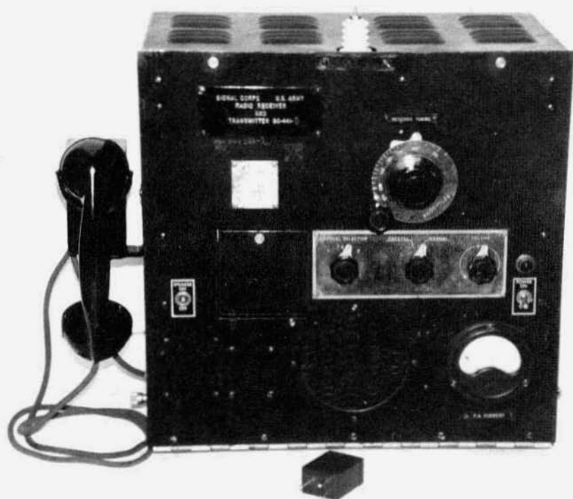
Fig. 1. Author's BC-441D. The large dial is RECEIVER TUNING. The three knobs in a row below this are (L-R) CRYSTAL SELECTOR (4 pos.), receiver CRYSTAL/MANUAL switch, and receiver VOLUME. The power on-off switch is on the left side of the front panel and speaker on-off is on the left. The four transmitter tuning capacitors are behind the fold-down door on the left, and the PA CURRENT milliammeter is lower right.
