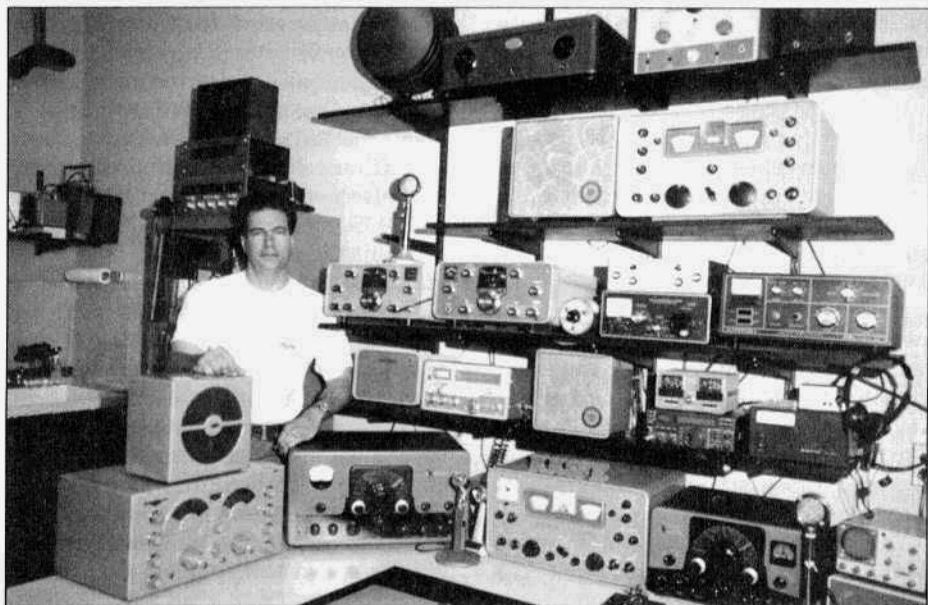
Keith Heitzmann, KK5FE, with some of his vintage gear. The two stations he operates mostly consist of the NC-173/Valiant pair on the lower left and the HQ-170/Ranger pair on the lower right.
