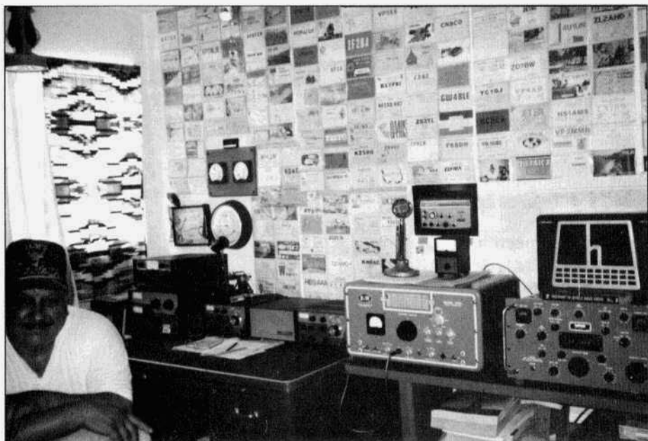
Earl Harris, K5FTE, in his vintage-equipped ham shack. His AM station consists of a B&W 5100 and an R-390A. The SSB equipment on the left side is a Drake C with an L4B linear.
