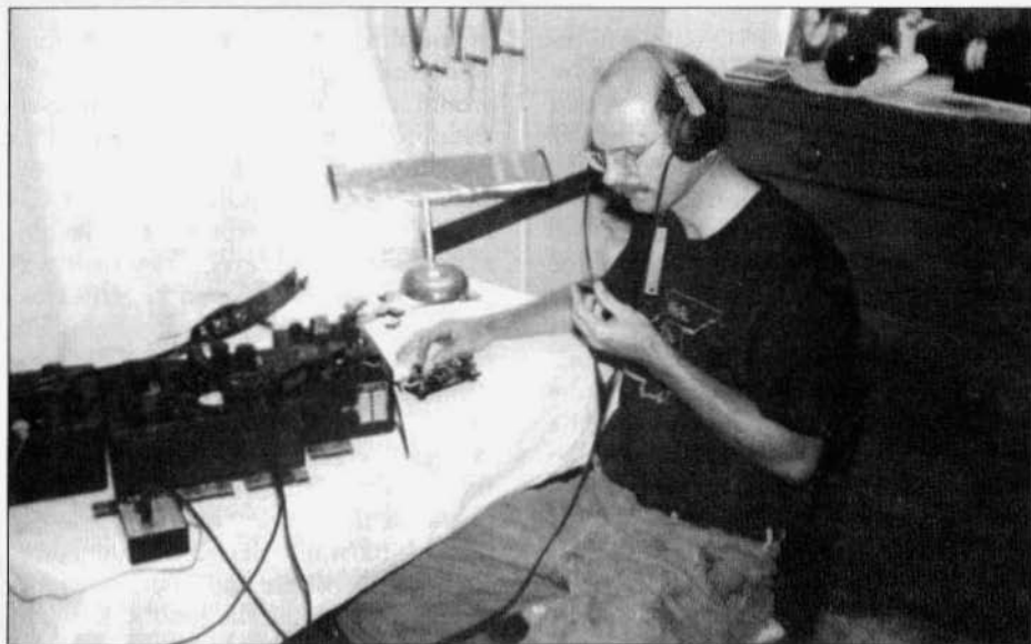
Eric Jones, N4TGC, operating his GRC-109 set. His GRC-109 set consists of the PP-2684 power supply, the R-1104 receiver and the RT-3 transmitter. The RT-3 is actually not part of the GRC-109 set but is the same as the correct transmitter the T-784 with the only difference being that it does not have code burst capability.
