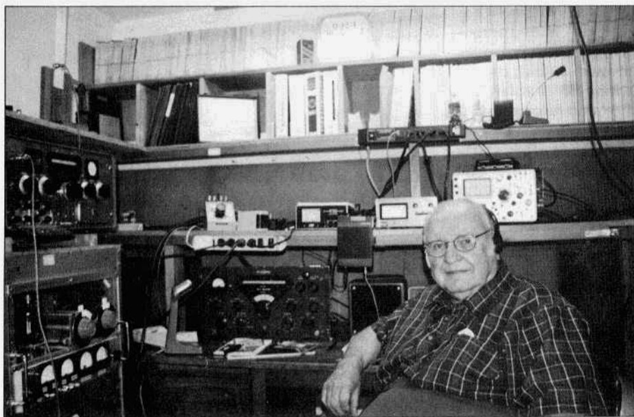
Louis W. Erath, W5BM, at his operating position. A CE 100V sits on top of a homebrew linear on the left and his receiver (on the desk) is a Collins 75A-2. He was first licensed in 1938 as W5HTO.
