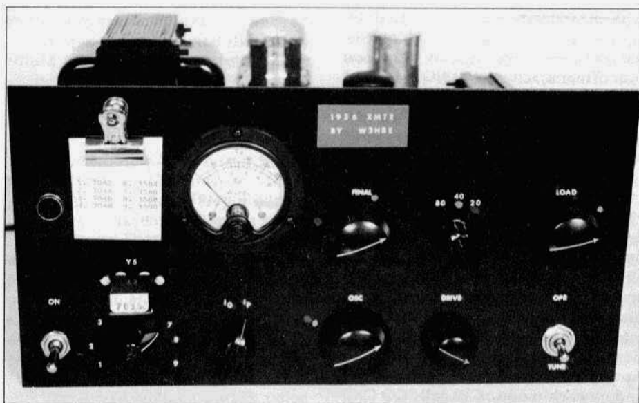
Front View - The '1936' AWA contest rig puts out 15W on three bands.
