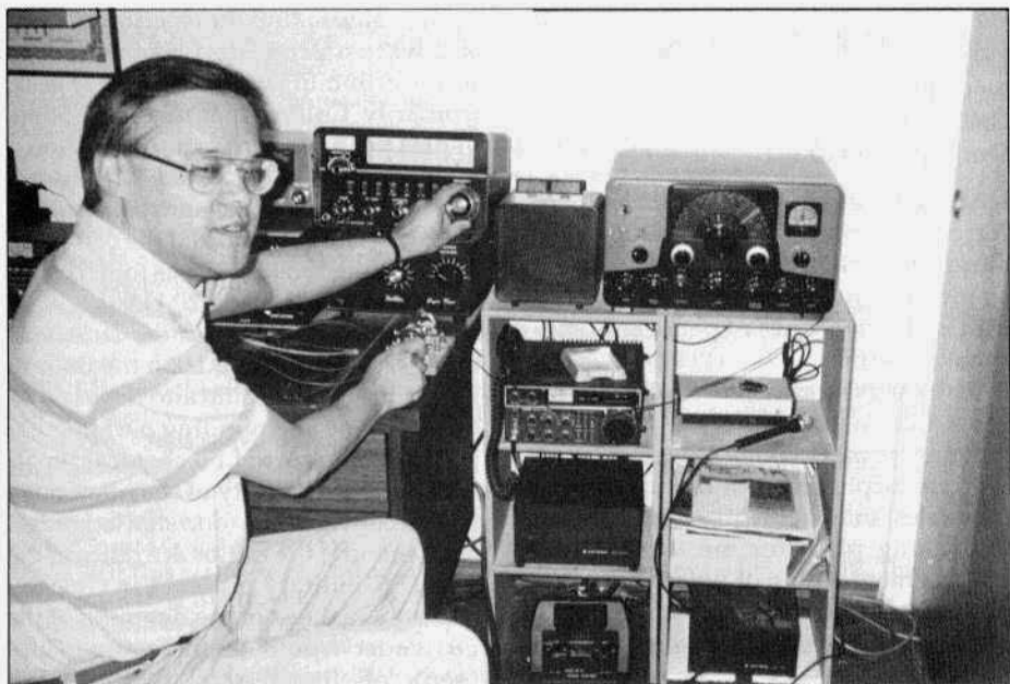
Mike Huey, W7ZI, with his vintage gear. The receiver is a Drake 2B and the transmitter is a Johnson Ranger. Mike operates on CW mostly.
