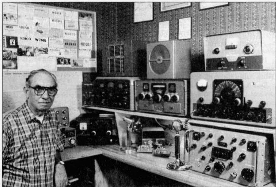
Gerald Morris, K6QY, with some of his vintage gear. For AM he uses the Valiant and SX-28. For SSB he uses the CE 100V with either the SX-28 or R-390A coupled with the CE Sideband Slicer. A Globe Matcher Sr. antenna tuner is shown sitting on top of the Valiant.
