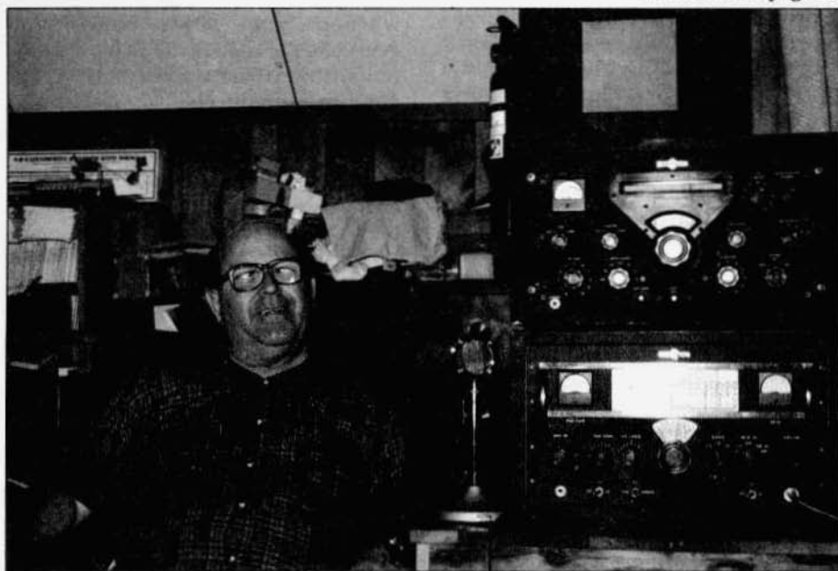
KØOJ at his operating position; Collins 32V-3 transmitter and 75A-2 receiver.
