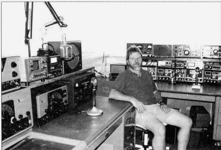
Michael McGinnis, N6TYF, in his vintage hamshack. His AM position, on the left, consists of a Desk KW, a Valiant, a Ranger, a Globe Scout and 75A-4 receiver. On the right side his SSB position consists of a Collins S-line, Swan 600 twins and a Swan 700CX.
