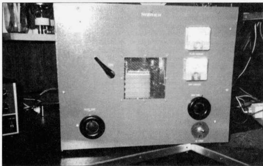
Front View of Flea Market Gallon. Lower left is output tuning, directly above is swinging link control. Right side is grid tuning with power switch just below. Grid and plate meters above.
