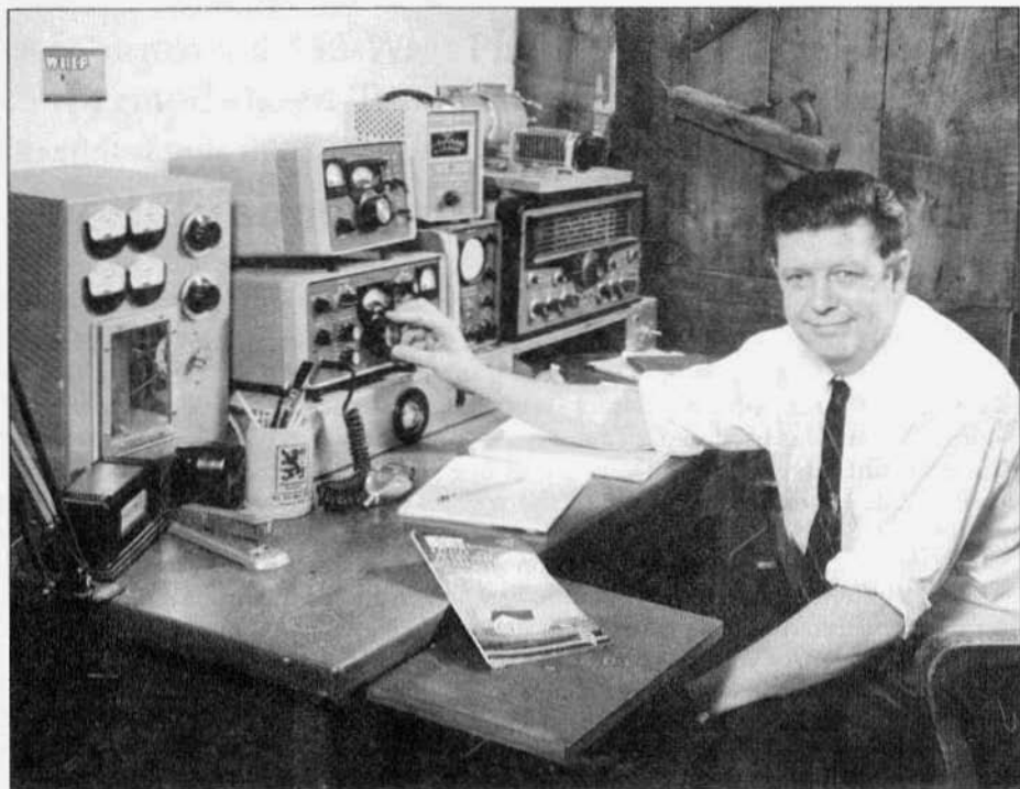
W1ICP in his hamshack in the mid-fifties. The amplifier on the left uses 4-1000s.
