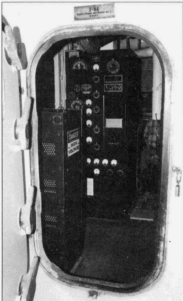
A TAJ (low frequency) transmitter visible inside Radio 2 on the cruiser USS Salem.
