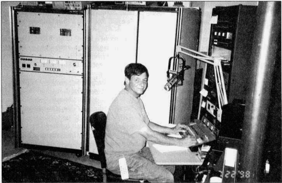
Mike Dorrrough, KO6NM/9, at his operating position. The transmitter on the left is a Collins 820D2 and on the right is a 820D1. He uses these transmitters on 160 and 75 meters. Mike is well-known amongst AM operators for his superb audio. Photo courtesy of Pat Keogh, WB9GKZ.
