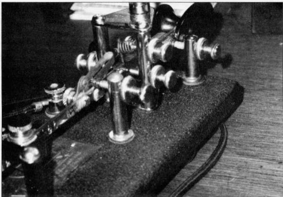
This photo shows the adjustment screws on an early Vibroplex bug.
