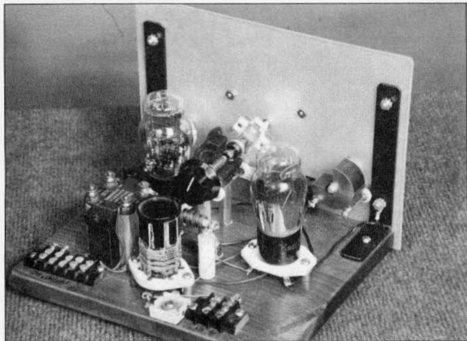
Breadboard receiver. Type 30 and 33 tubes. This receiver circuit was featured in "How to Become a Radio Amateur" back in the mid-30's. The most difficult part to find was the double-ended tuning capacitor. Note main tuning knob in front of the coil. The bandspread dial on the front is a National 'Velvet Vernier'.
