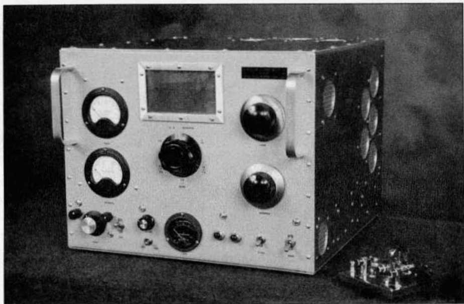
Front panel was sanded, primed and sprayed with ordinary spray can enamel. Center black-face meter is the old standard 'Monimatch.'
