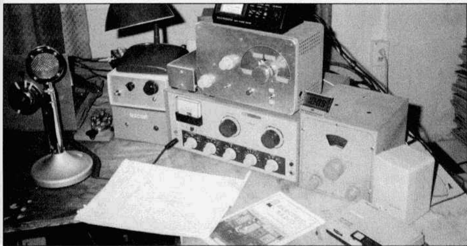
The 'Mighty Midget' is paired up with a DX-60B at N2CQR. This station is used on 40M AM. Note the Radio Shack computer speaker on the right. On the left is a solid state HB QRP station for 20M CW.
