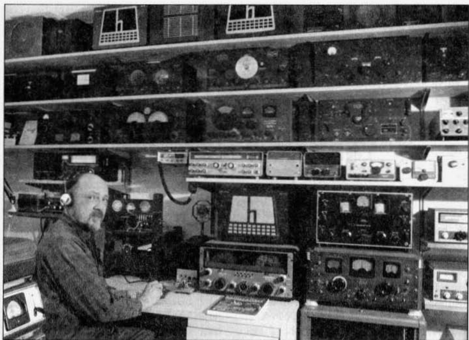
The author's shack in 1997. The restored high-C Hartley transmitter is in front of the author. Note that the Hallicrafters 5-T and SX-15 are the same receivers that appear in the 1937 photo of W8CPW's shack.
