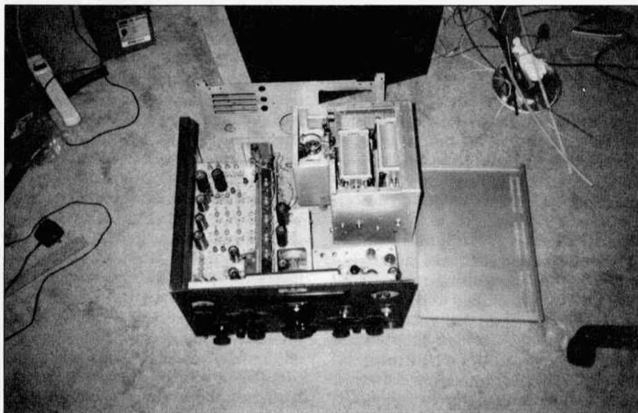
Exciter is readied for installation. Note gold colored side cover which was also alodined before outer portion was painted the familiar Saint James Gray.
