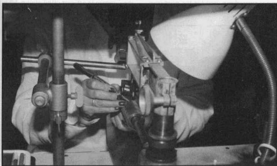
Winding of mesh filament for the Svetlana 3CX3000A7 & 4CX10,000C.
