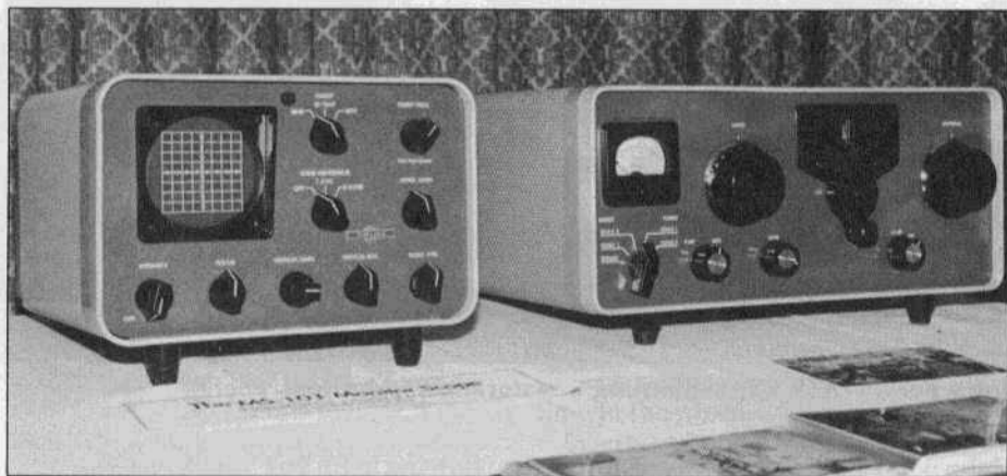
On display at the convention, left, Jay Miller's, KK5IM, SC-310 Heath to Collins spectrum scope conversion and on the right Butch Schartau's, KØBS, antenna tuner built in a Collins case. Photo by Gene Duprey, K1GD.
