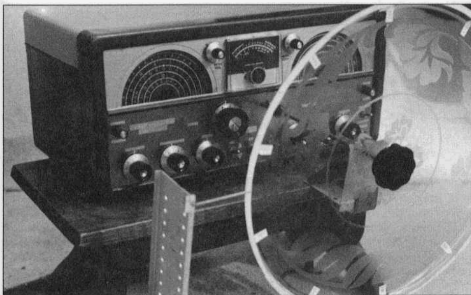
The author's 'Rube Goldberg' setup consists of an 18" dial (a plastic serving tray) and a 9" extension shaft.
