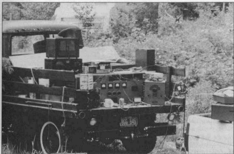
A vintage truck (1960 Willys) carries the vintage radio gear. The 'flagship' transmitter was the Meissner 150B shown front and center in the back of the truck.
