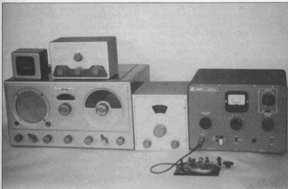
Mike Langner's, K5MGR, reassembled first station: NC-57 with Heath QF-1 Q-Multiplier and very rare SM-57 S-meter; Knight T-50 transmitter with Heathkit VF-1 VFO and J-38 straight key.
