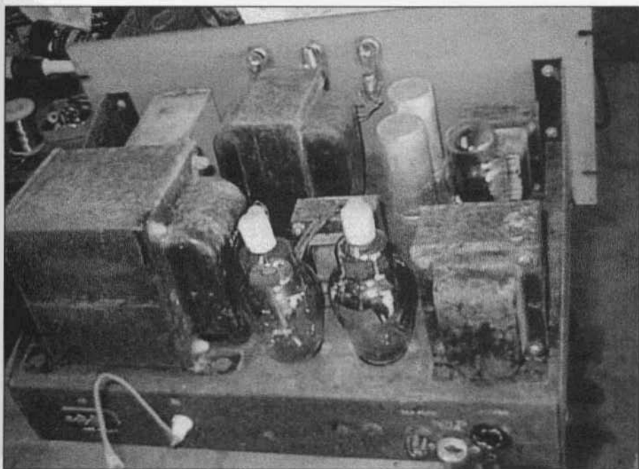
Look at the rust on the HV power supply
