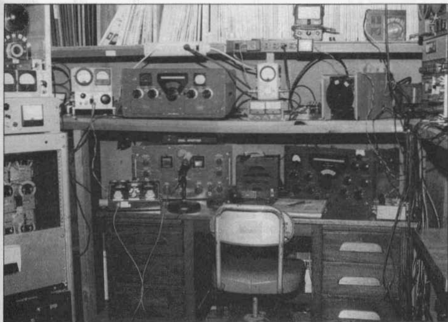
The author's operating position showing speech amplifier and compressor to the left of the Heil Goldline microphone. The CE 100V on the shelf is used as the RF driver. The modulator is to the left of the 100V.
