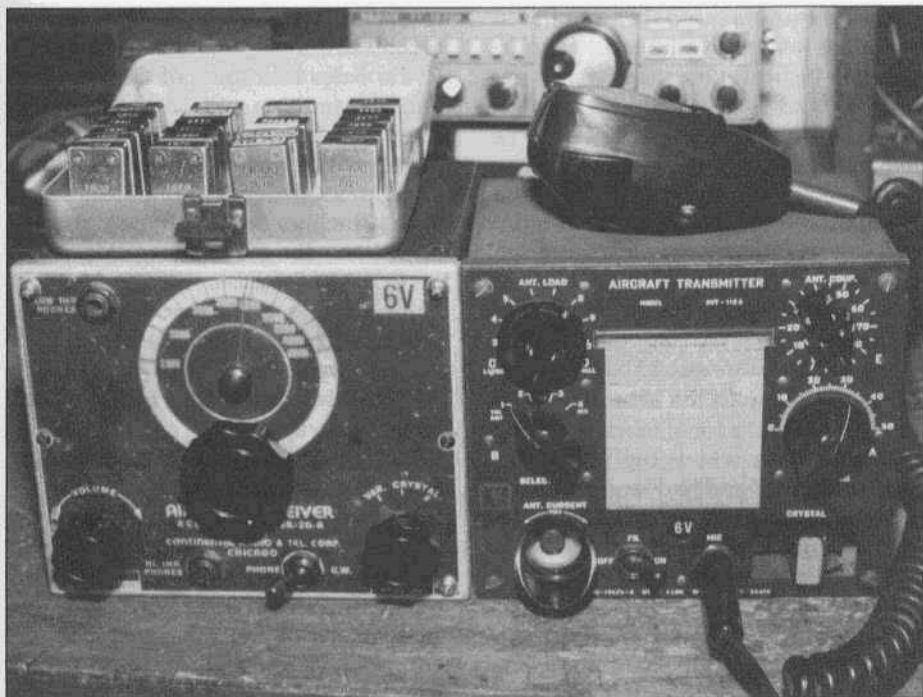
RCA AVR-20-A receiver and AVT-112-A transmitter. Note government inspector's stamp above and to the left of the tuning eye tube.
