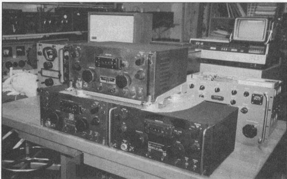
The author's 3 R648/ARR41 receivers. Notice the shock mounts on the top receiver and the R-390A in the rear for size comparison.
