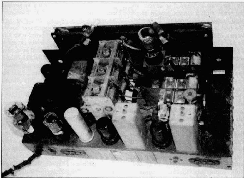
Looking down on the Howard 436A chassis. The open holes on the right end of the chassis are for the second 6SK7 and IF transformer of the 437A.
