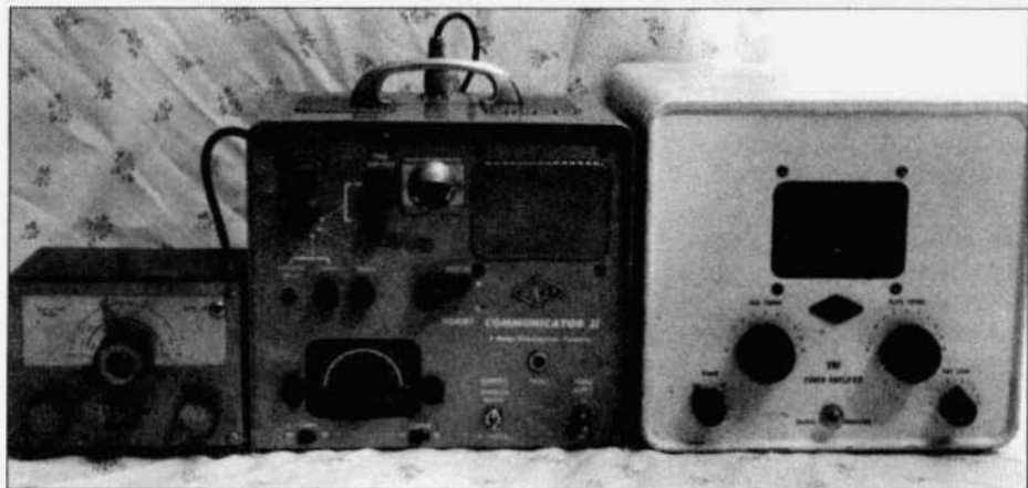
Gonset Communicator II with the matching VFO on the left and 50-watt amplifier on the right.
