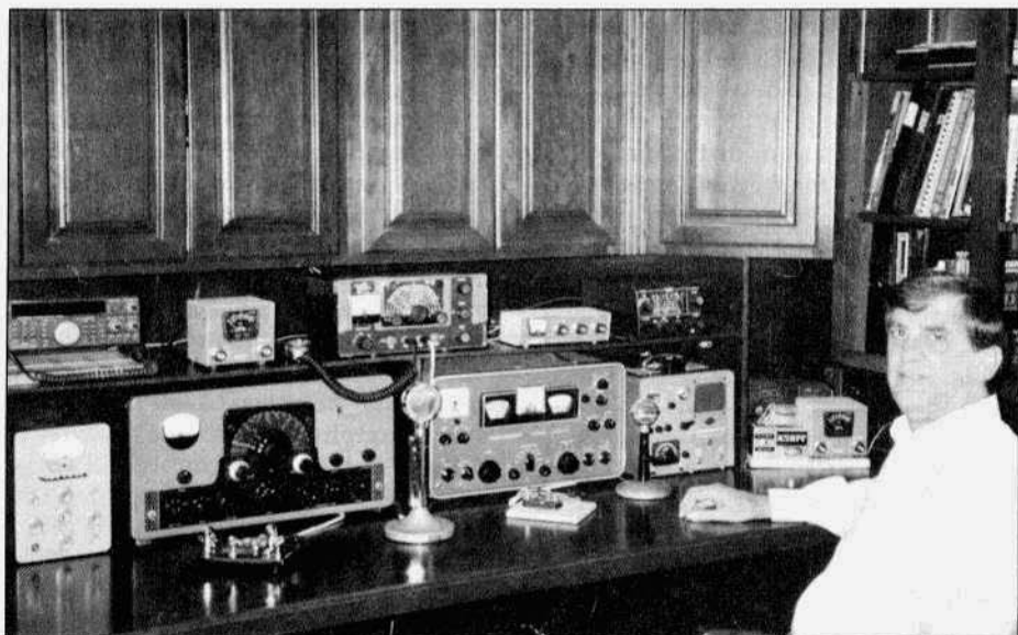
Tom Anderson, K5HPF, his Viking Valiant, Hammarlund HQ-170A and Heathkit SB-10 sideband adaptor. Note Heathkit SWR meters and phone patch.
