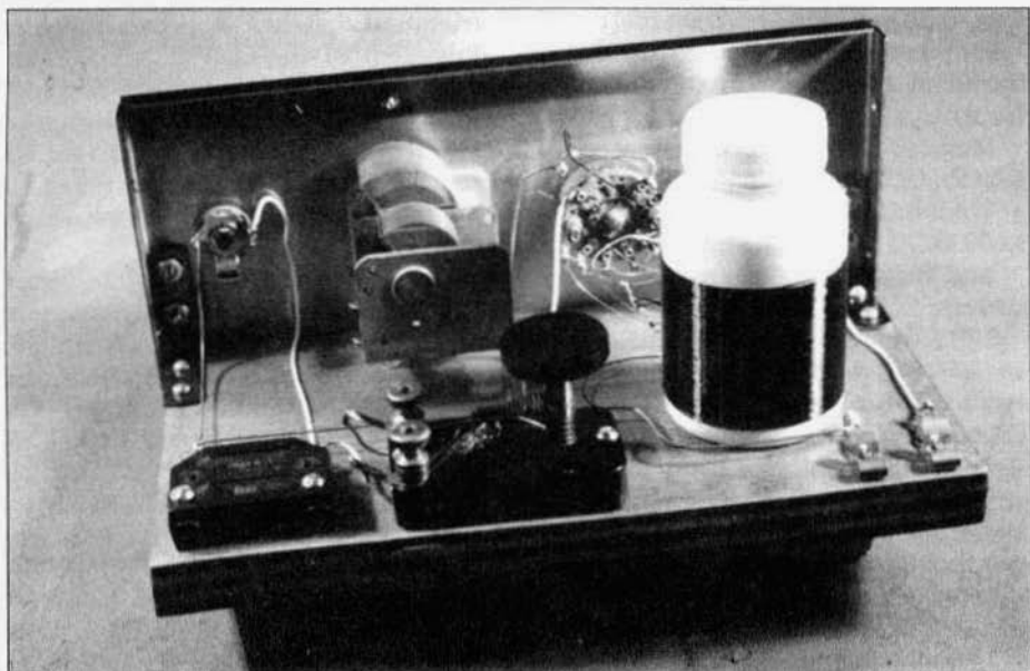
Figure 8. Rear view of crystal set showing the Murdock detector.
