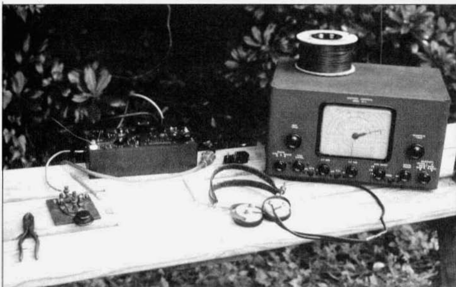
W4MEW's VFD station consisted of a SST-1 OSS transmitter and a Echophone receiver.
