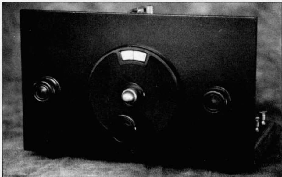
The front view of a 2-tube receiver. It covers from the broadcast band to 30 meters using plug-in coils. The vernier dial is a National from the 20's.
