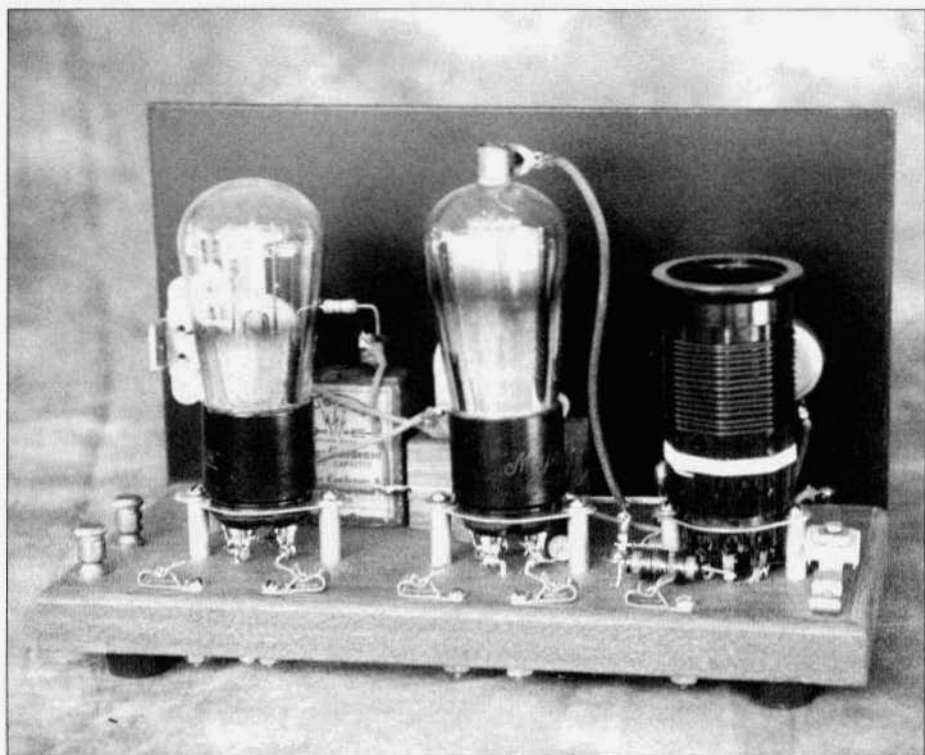
This receiver uses a 224 detector and a 227 amplifier.
