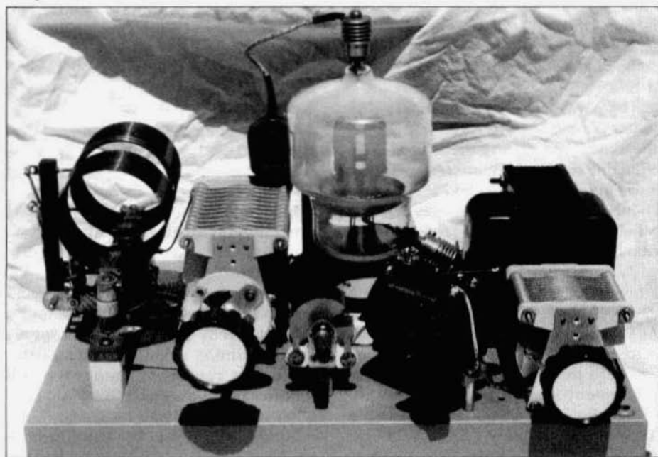
Amplifier with 304TL. Notice the smoke inside the tube.
