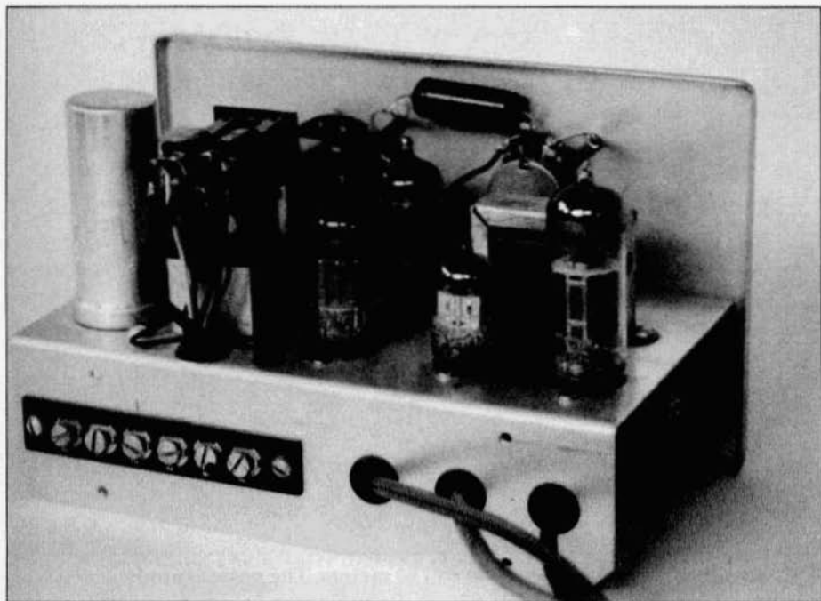
Behind the panel of the VX-1 you will find a lot of hollow state electronics.
