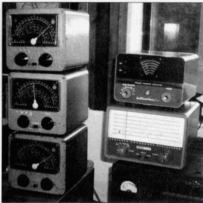
The VFOs tested. The three on the left are Globe 755s. The Hallicrafters HA-5 is on the top right and the EICO 722 is in the lower right.
