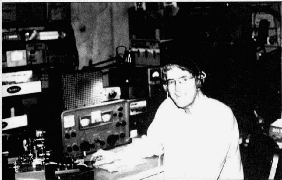
Jay, W7JWA, with his homebrew station. Besides the xmtr and rcvr he also built the keyer, a paddle and a hand key.
