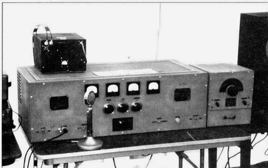
Dale Gagnon, KW1I's Meissner 150 (U.S. Signal Corps transmitter Type 02520 and matching exciter unit Type 02433)
