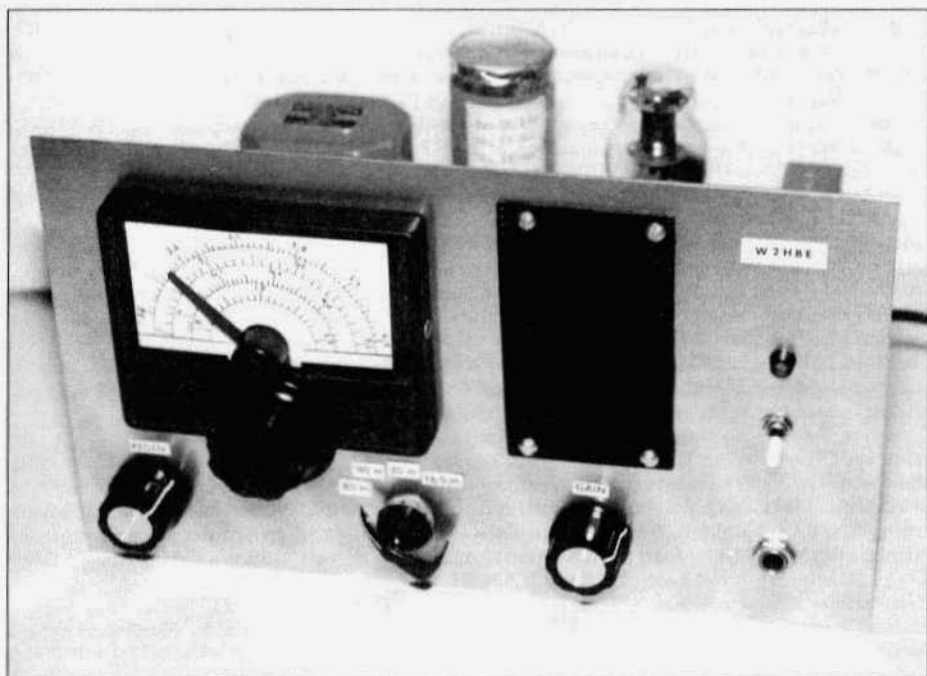
Fig. 1. Front view of the bandswitching regen. Speaker grill is perforated with ten .07 inch holes per inch.
