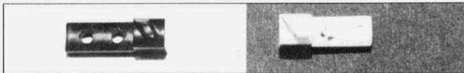
Figure 7. The old thread follower on the left and the brand new part on the right.
