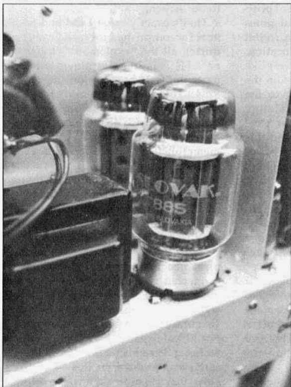
The modulator tubes in the author's Ranger are KT88s
