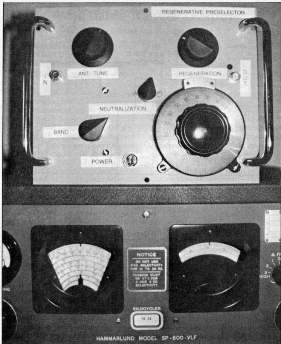
The regenerative preselector sitting on top of the author's Hammarlund SP-600-VLF receiver.
