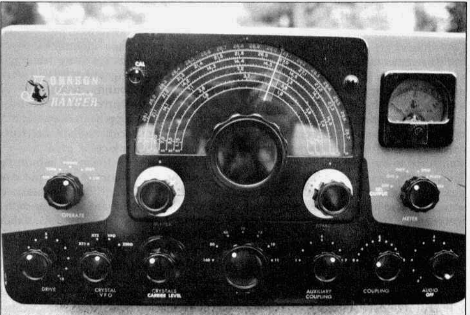
Figure 3. The Front panel of the modified Ranger. Note the new controls—Carrier Level and Cal.
