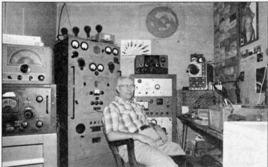
This is a photo of Les Lester, K6HQI who ran the 14.286 AM net for over 20 years. The homebrew transmitter behind him ran a pair of 833As modulated by 833As. The receiver he used and his yagi antenna were also homebrew. He passed away 5 or 6 years ago.
