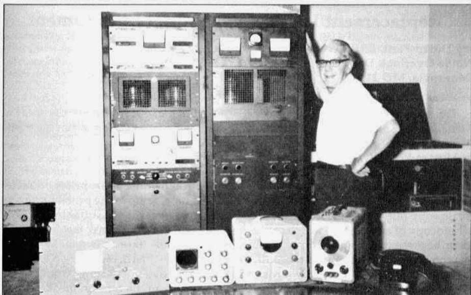
'Hoisy' Hoisington, W4CJL. On the back of the photo he has written, "Hi there Rick: Appreciate ur interest in Advanced Modulation. This is our "Standby" xmtr, 1 KW output, 4-1000As modulated by pr 4-1000As. Built it up from scratch about 7 years ago. Uses ultra-modulation, only 125% positive peaks." There wasn't a date on the photo but it's probably 20 years old.
