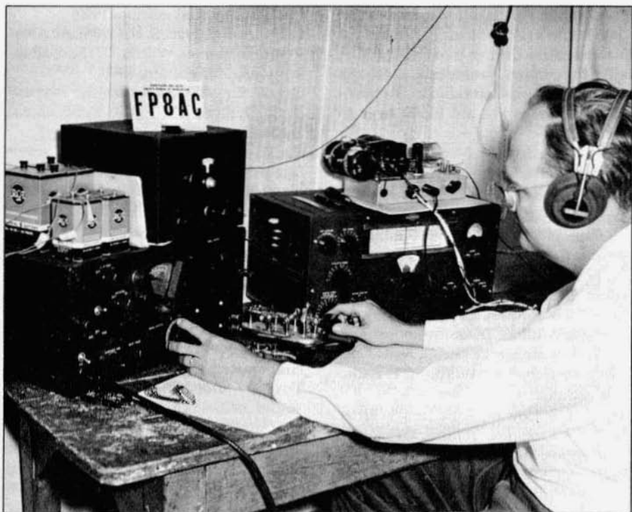
W6SAI/FP8AC operating in the Saint Pierre & Miguelon Islands July 7, 1950. The receiver is a BC-348 (one of his favorites) and the exciter is a Collins 310-B5. See October 1950 CQ, page 31.
