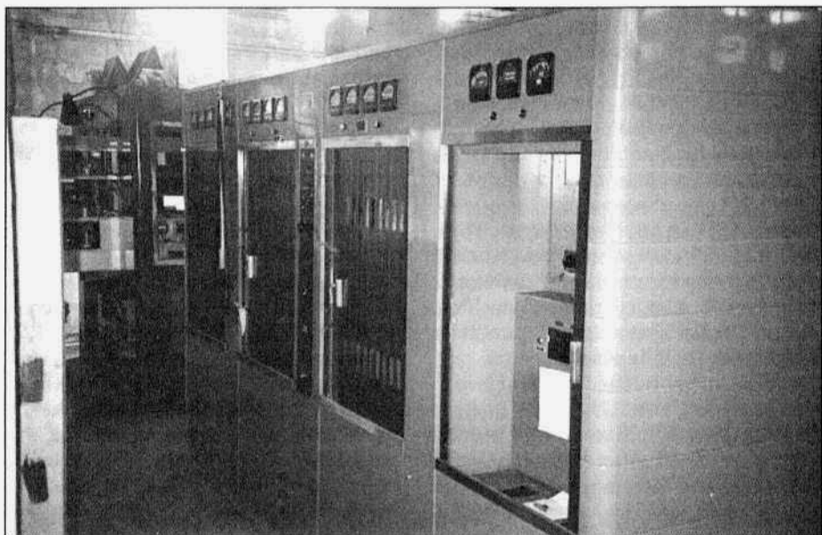
RCA transmitter 303L in operation on 20m. During its lifetime this 50s vintage transmitter has been used for point-to-point service (in AM mode), Teletype and finally for CW. In the background an RCA H set may be seen undergoing restoration.
