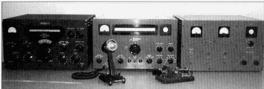
The author's Eldico station: Collins 75A-4 receiver on left; SSB-100F transmitter center and SSB-1000F amplifier (the subject of a future article) on the right.
