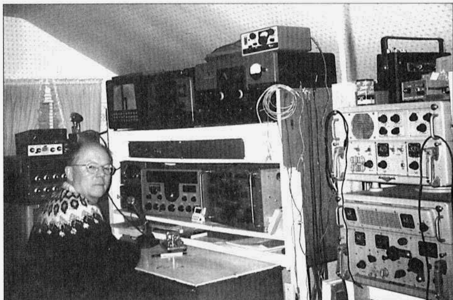
Dennis Olmstead, WB9EMD, at his operating position. On the right side of the photo is the rare 68-tube National receiver, the URR59A. The bottom piece is the RF deck and the top piece is the IF and SSB deck.
