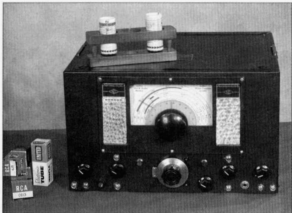
Completed receiver with coil holder and coils. Note coil identification stripe on left aluminum panel.
