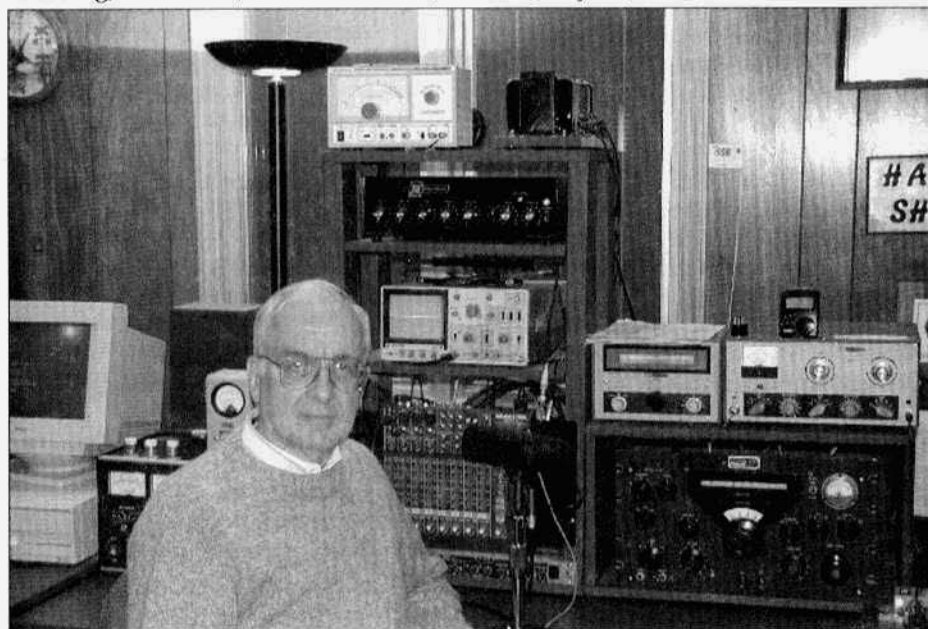
Ken Barber, W2DTC in his ham shack. The DX-60B (which he runs into a linear amplifier) is his main AM transmitter. He also uses an external modulator.
