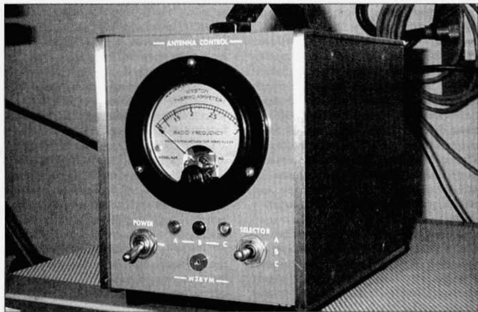
The antenna controller is housed in an HP VOM case.
