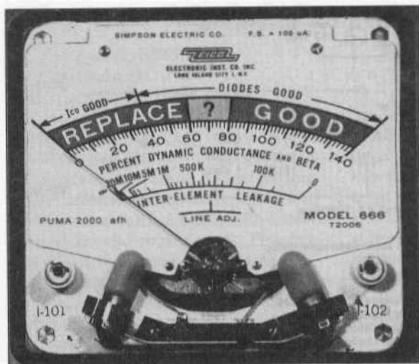
Figure 2 is a photograph of the meter with its cover removed and the replacement face.
