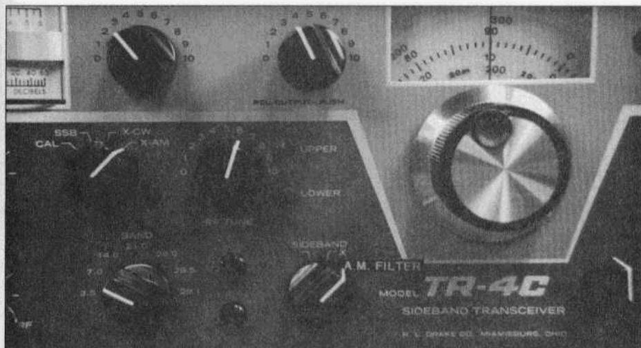
Front panel of the Drake TR4CW transceiver. Note the AM position on the sideband switch where the CW position was originally.
