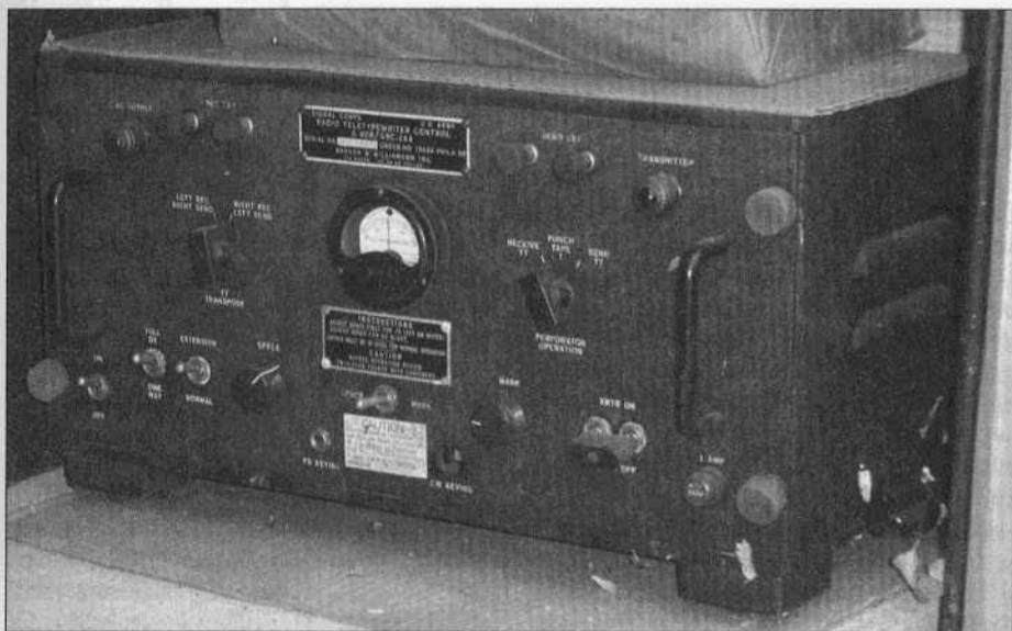
Figure 4. The C-808/GRC-26A Radio Teletypewriter Control. The manual describes this unit as the 'Control Center' of the entire system.
