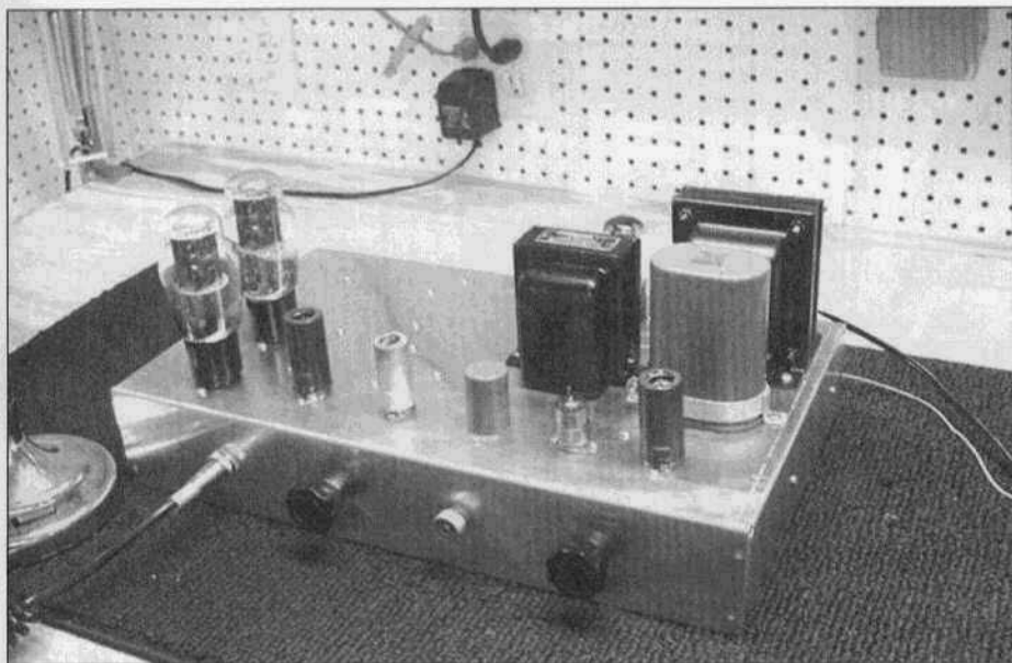
Top view of speech amplifier showing power supply on right and 6B4G triodes on left.
