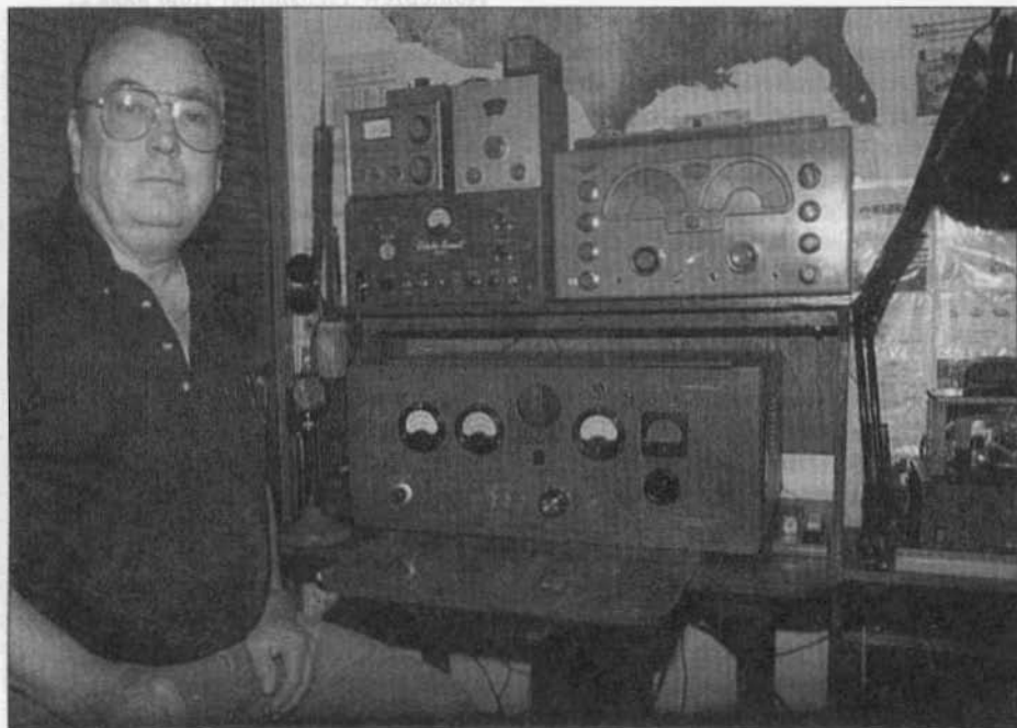
A recent photo of Fred Pfannenschmid, WØZZS, in his vintage ham shack. The transmitter in front of him is an HT-9 he purchased used in 1956. Above the HT-9 is a Globe 65-A and an NC-173. More on the HT-9 below.
