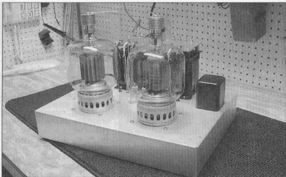
Front of modulator chassis showing 4-1000's, filament transformers and driver transformer.
