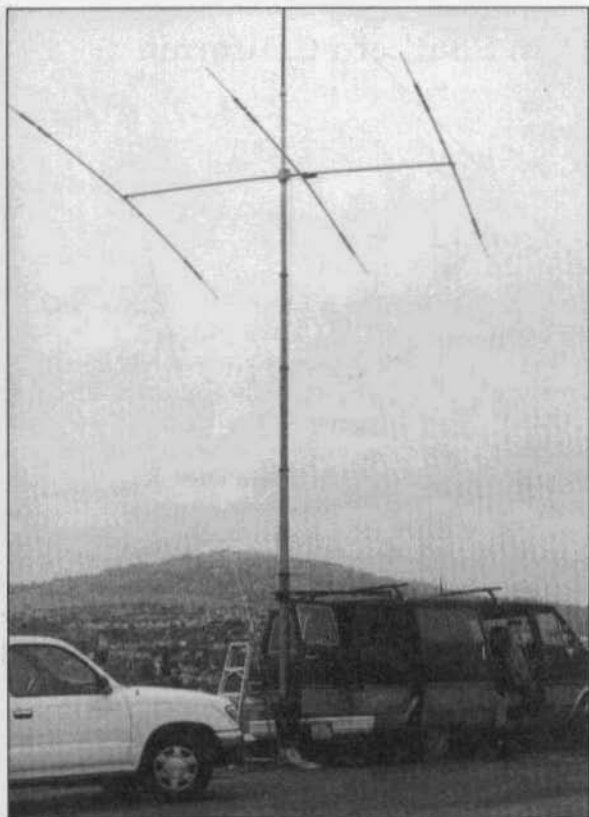
A tri-band yagi is held aloft by a 30-foot military surplus pump-up mast. An end-fed 130-foot wire was used on the lower bands.
