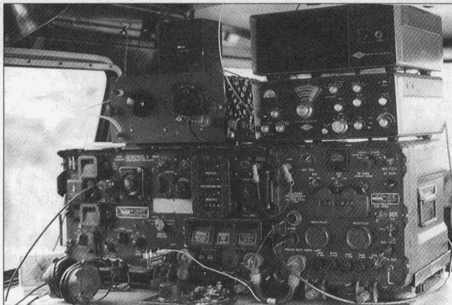
Equipment inside the author's van: T-195 (lower left); R-392 (lower right); Gonset G-76 (upper right).
