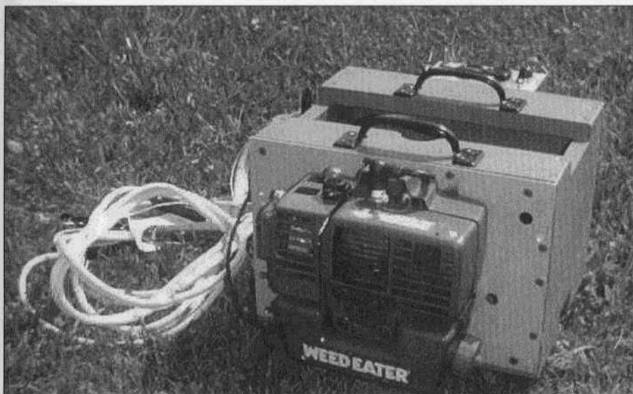
Front view of the Weedeater-powered generator
